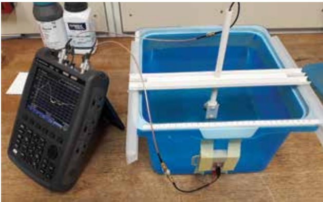
Figure 3. Measurement setup for implantable to on-body channel measurements on a muscle tissue equivalent liquid phantom.
