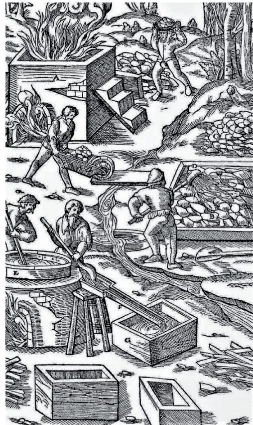
A – furnace, B – enclosed space, C – aluminous rock, D – deep ladle, E – cauldron, F – launder, G - troughs
