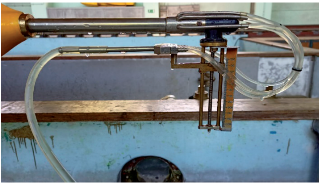
Fig. 3. The five-hole Prandtl Pitot tube installed at the stern.
