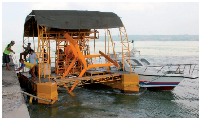
Fig. 12. BRIN vertical-axis ocean current turbine prototype conducted in 2014 (BRIN-documents, 2014)
